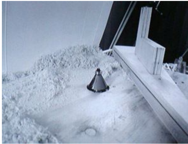
Tapered router bit for shaping cone segments
