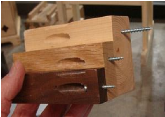
Typical pocket hole screw location at midpoint of material thickness
