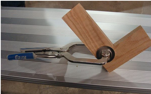
Kreg Clamp used to secure and align joint surfaces
